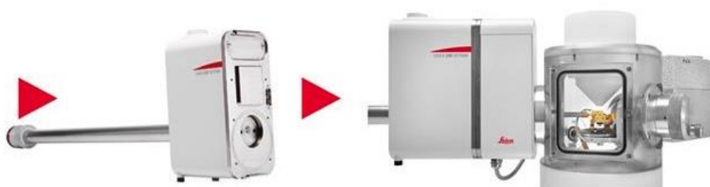
Figure 7.7 - Sample transfer system produced by microscope manufacturer Leica (left) The samples can be loaded into transfer system under clean, inert atmosphere or vacuum conditions. The sample transfer device can then be attached to a compatible docking chamber attached to various compatible instruments and the sample transferred without exposure to unwanted contamination
